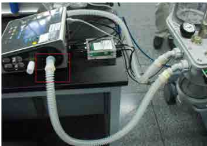
FIGURE 4-22 Pneumatic connection with the calibration device (VT Plus)
