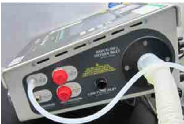
FIGURE 4-42 Pneumatic connections with the calibration device (VT-Plus)
