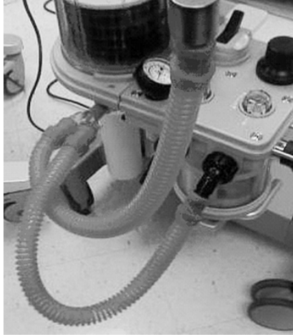
FIGURE 3-25 Vaporizer Leak Test Setup
